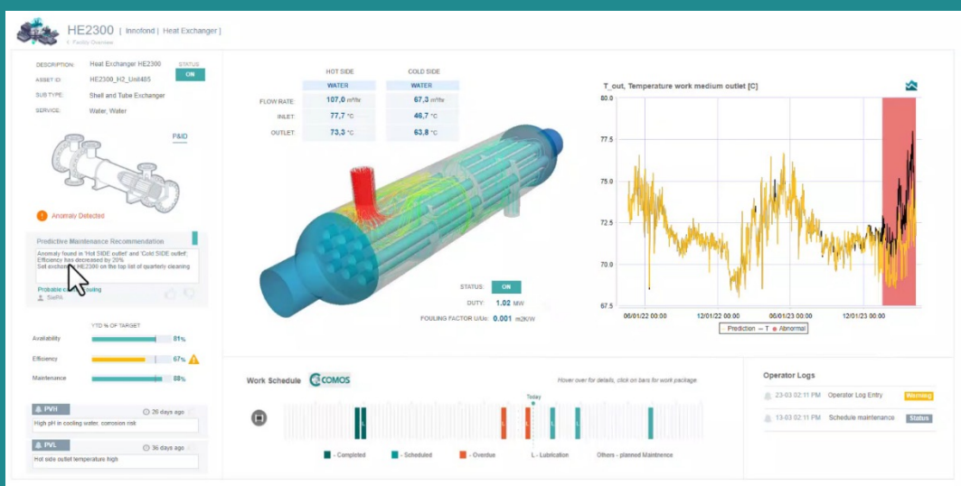
Figure 19 - Predictive maintenance recommendations: understand that your heat exchanger lost efficiency
